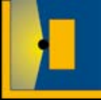
Narrow beam linear spotlighting of architectural feature.
