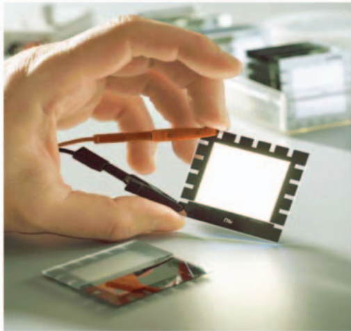
Figure 8 A warm white coloured OLED research sample measuring 35\text{ mm}^2 \times 35\text{ mm}^2 (Photo: Philips)
